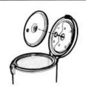
To close the outer lid, simply lower it until the lid latch engages with the lid catch with click.
